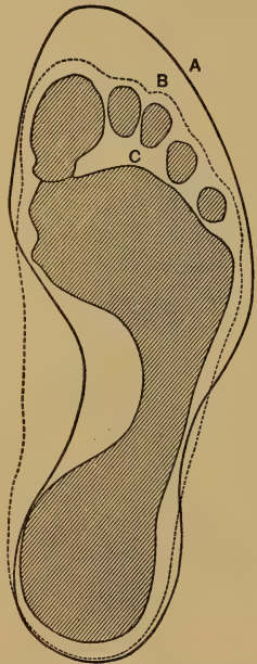
The proper relation of the sole to the shape of the foot: A, outline of sole; B, outline of foot; C, imprint of foot.
